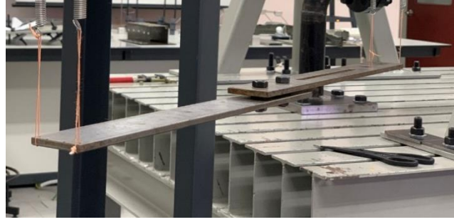
FIGURE 2. Experimental set-up of bolted structure
