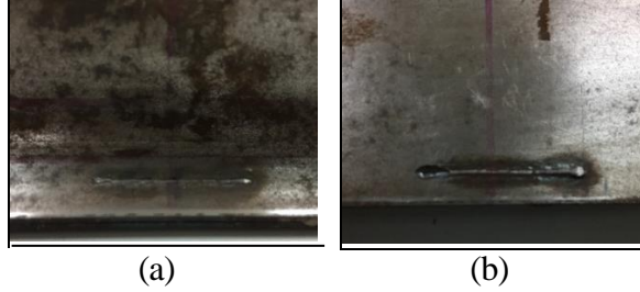
FIGURE 12. Welded area with HAZ on (a) hat component, (b) flat plate component
