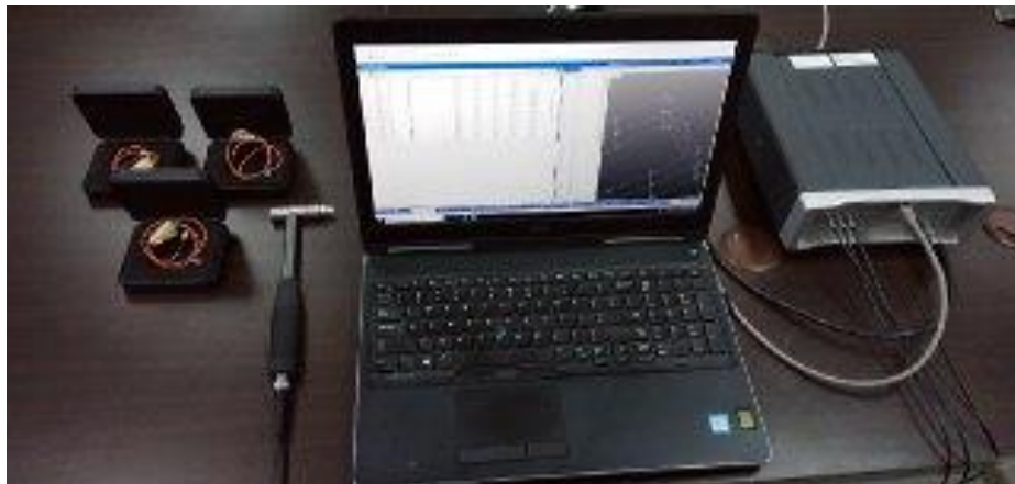
Figure 2. Testing equipment for experimental modal analysis
